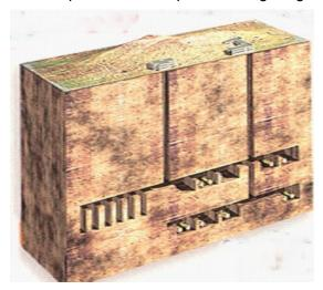
Figure 18: Artist's view of underground waste depository showing service buildings and shafts, and storage caverns.
