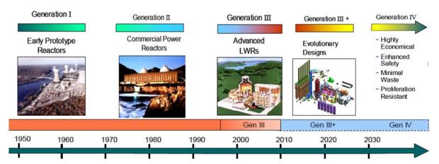
Figure 14: Timeline for evolving reactor generations Gen I – Gen IV characterized by improved operational and proliferation safety at reduced waste, In some countries, Gen III+ reactors are already under construction, ahead of this schedule (Adapted from DOE-Gif.)
