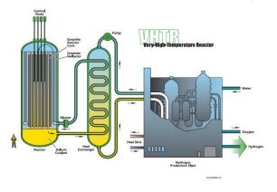
Figure 15: VHTR concept with (left to right) reactor vessel with graphite core and reflector, heat exchanger, and on-site hydrogen plant. (From DOE-GIF, 2002)
