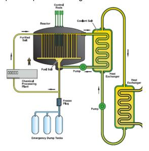
Figure 20: Schematics of a molten-salt reactor.
