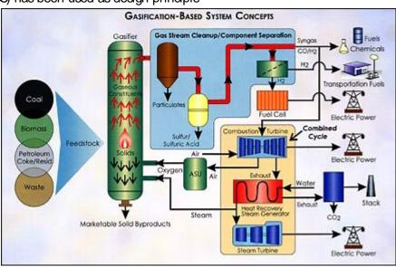
Figure 2: Schematic flow diagram of IGCC coal power plant with hydrogen and synthetic fuel production, as well as carbon dioxide capture (DOE, 2003).
